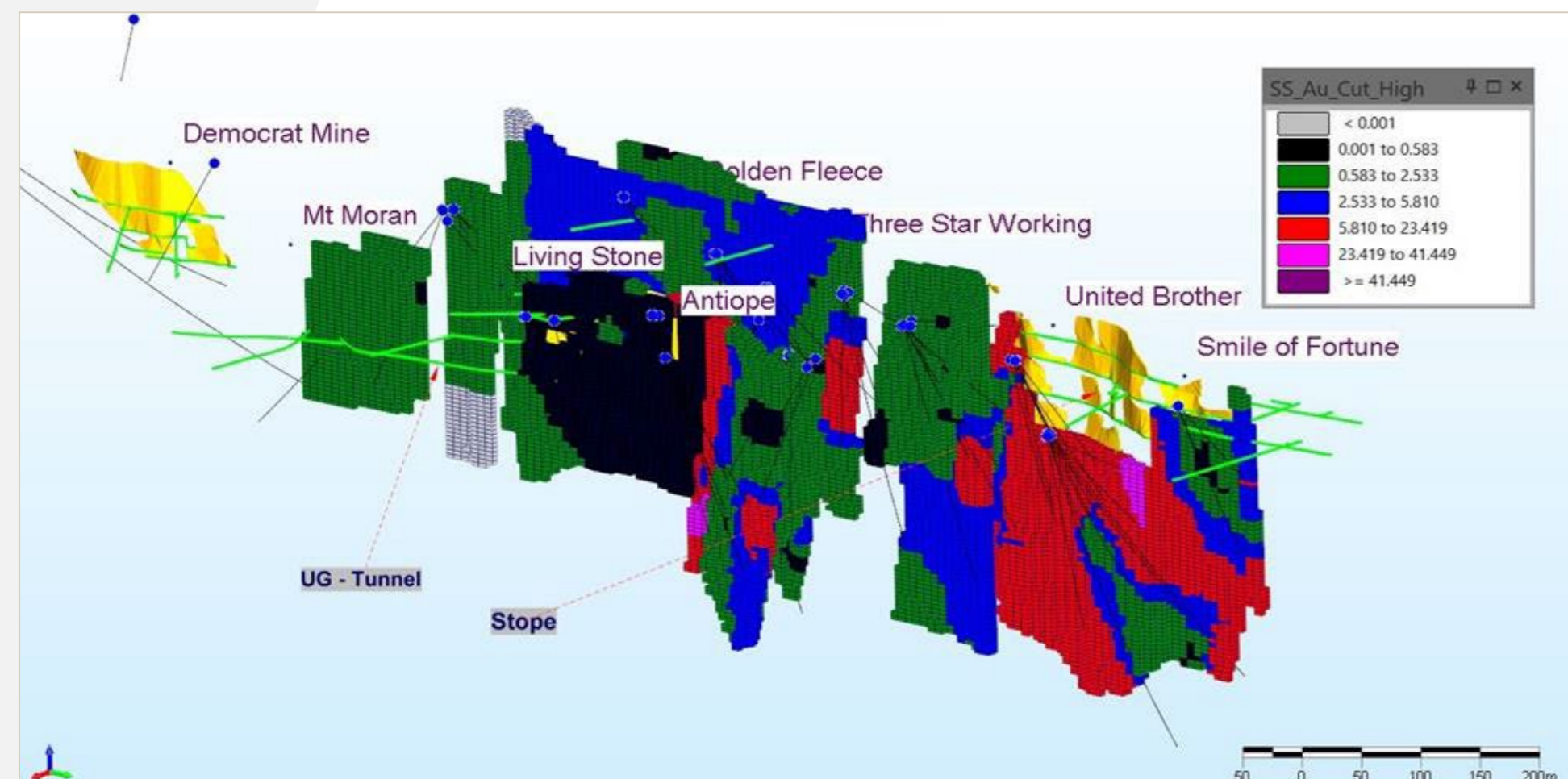
Figure 2 Representative long-section showing 3-D block model of Au distribution, historic tunnels, stopes and drill hole locations at Sunnyside (legend in g/t)
